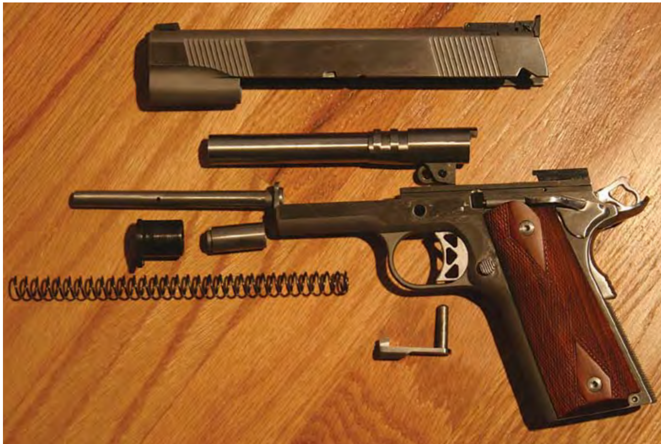
(above) Pointman field stripped for complete cleaning. This handgun is a complete John Browning 1911 design.
