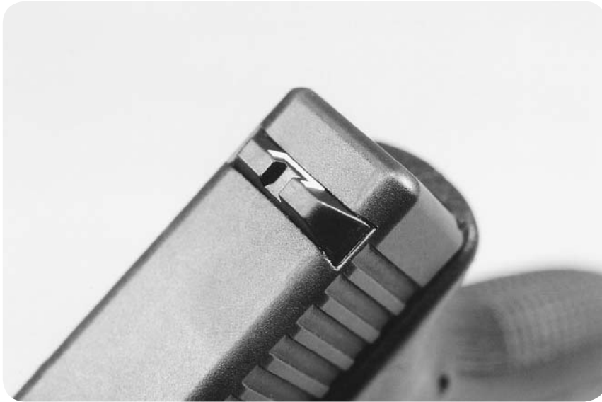
The rear sight in its dovetail.
