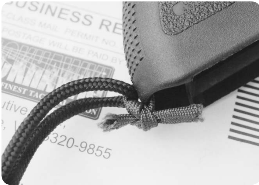
The Blackhawk Industries lanyard tied to the Glock frame with 550 cord. The next step is sealing the ends with a match or lighter.
