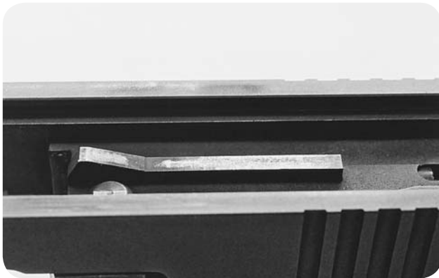
The cartridge pickup rail. On the Glocks in .45, the rail should look like this, with an angle in it. If yours doesn't, have Glock upgrade it.
