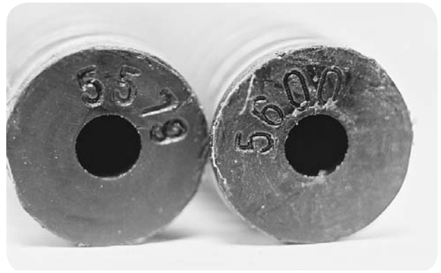
Glock recoil spring assemblies are marked. The 5600 on the right is for a G-21. The 5579 on the left is for a G-22.
