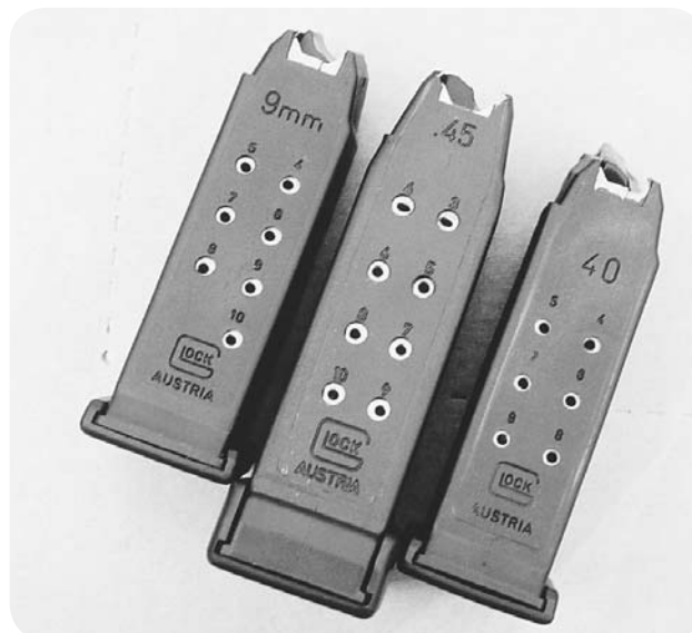
Increasing the capacity of compact models makes the magazines a lot longer.
