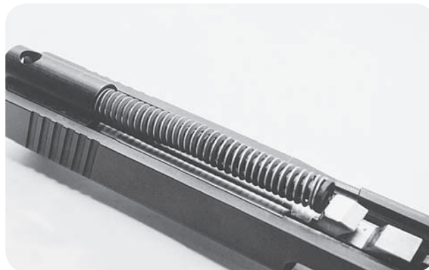
Despite the extra length, the slide uses a standard Glock recoil spring assembly.
