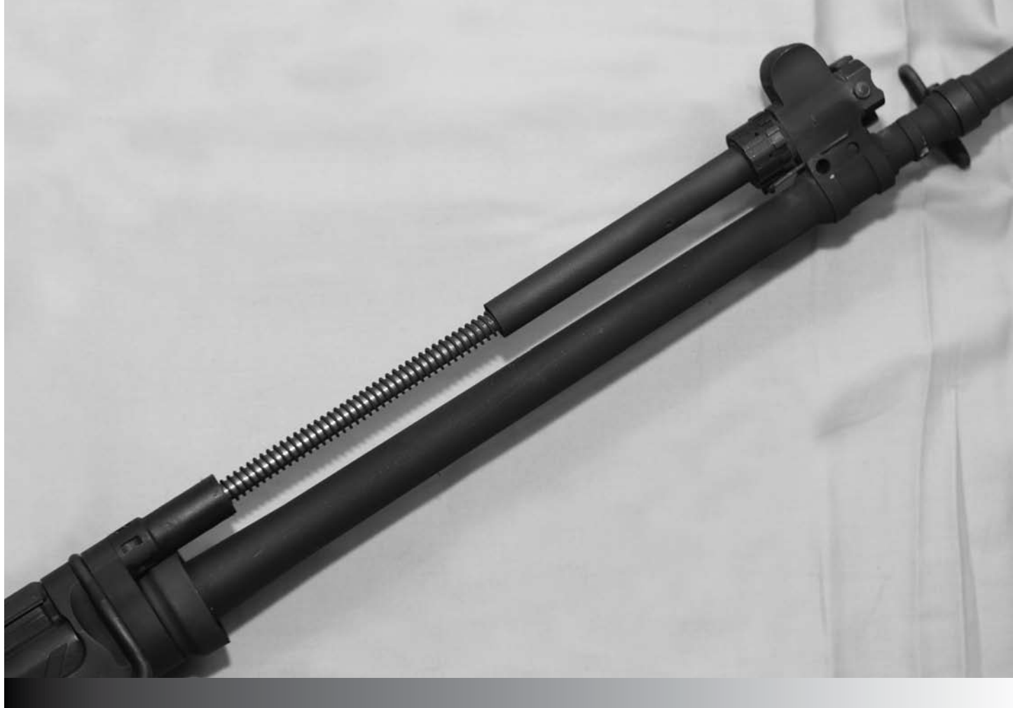
The FAL gas system has a return spring and depends on the user for proper gas flow.
