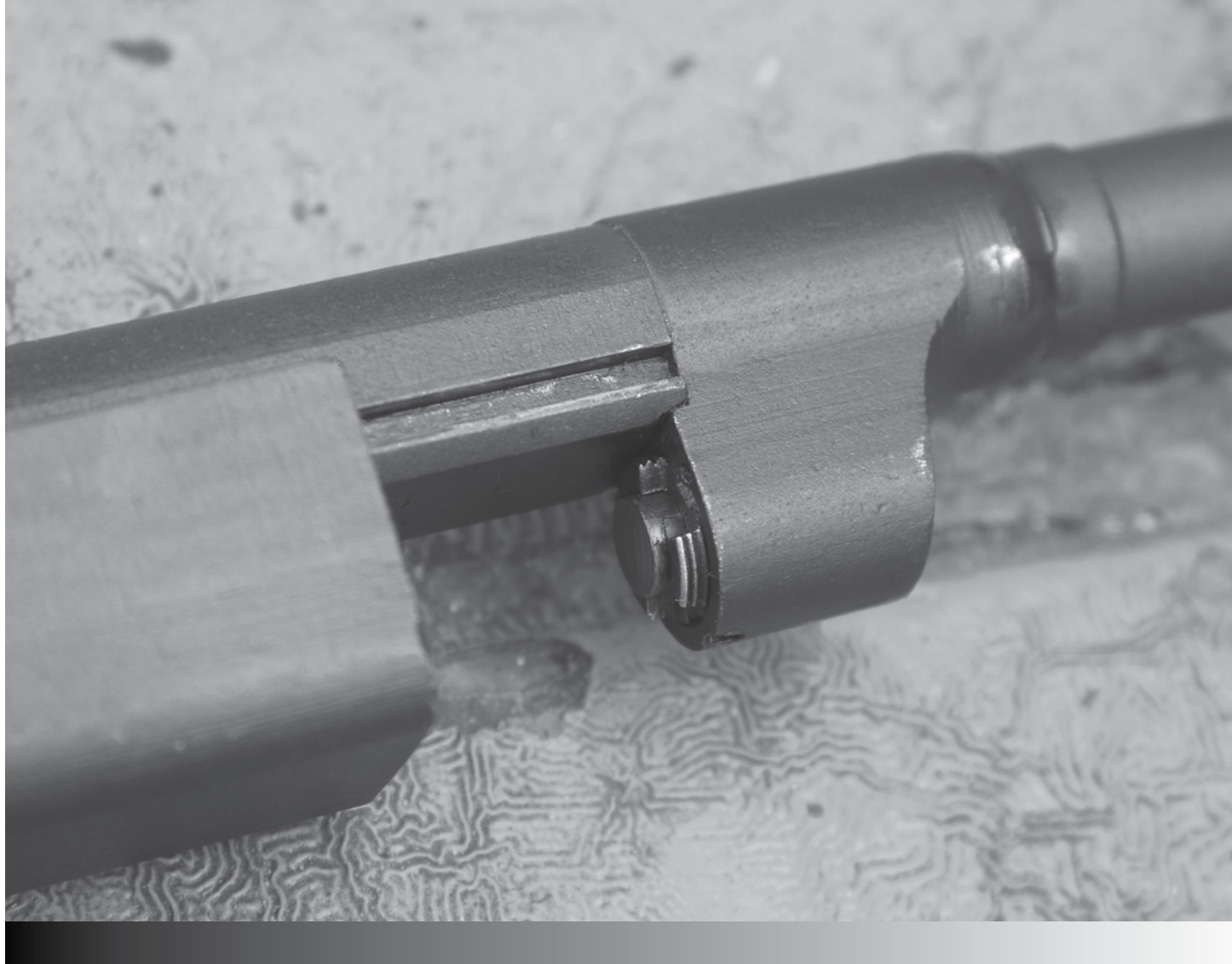
The M1 Carbine is a short-stroke piston design.
