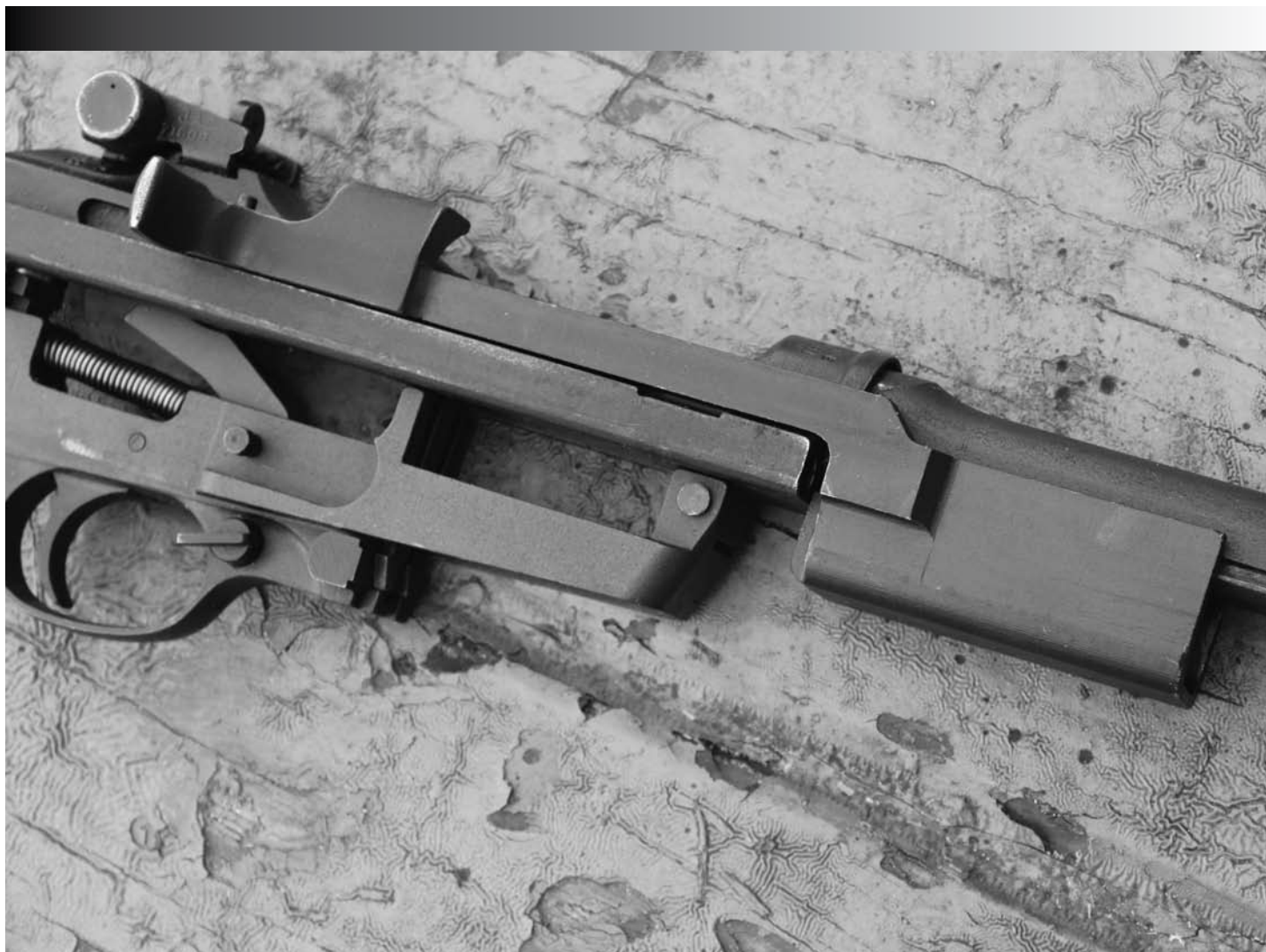
The piston launches the carbine op rod, which turns and cycles the bolt, returns and chambers and locks. All very simple.
