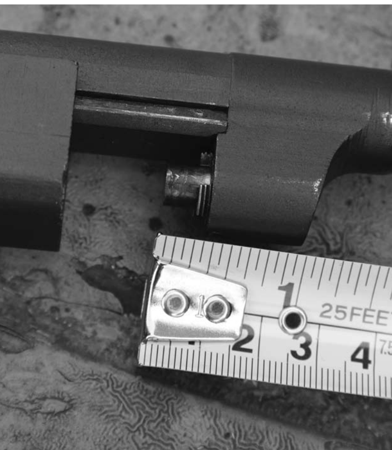
The M1 Carbine piston snaps back and forth maybe a quarter of an inch. That's all it needs to do to drive the system.
