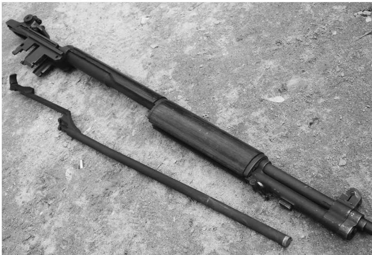
The M1 Garand is a long-stroke piston system. The gas works on the muzzle end of the op rod, which works the bolt. No parts in between.
