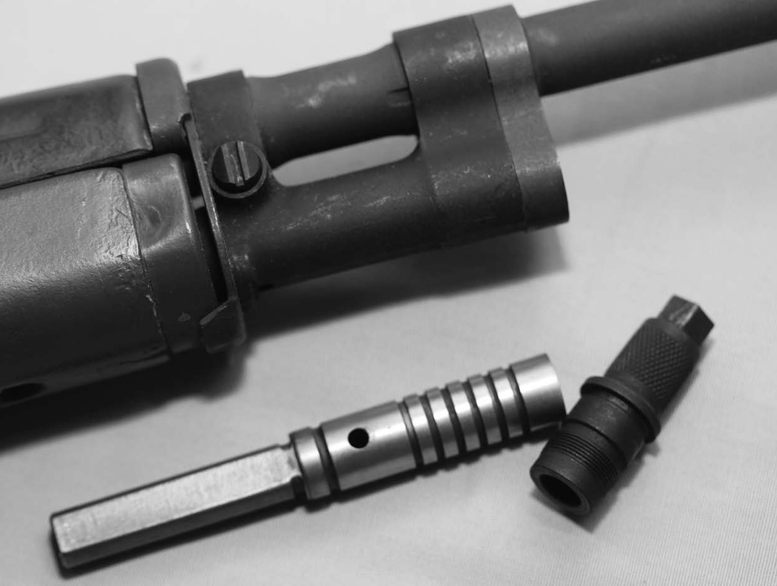
The M14/M1A piston has a vent hole in it. When it lines up with the gas port, gas flows. As the piston moves it closes off the gas flow, thus acting as a self-limiting system.
