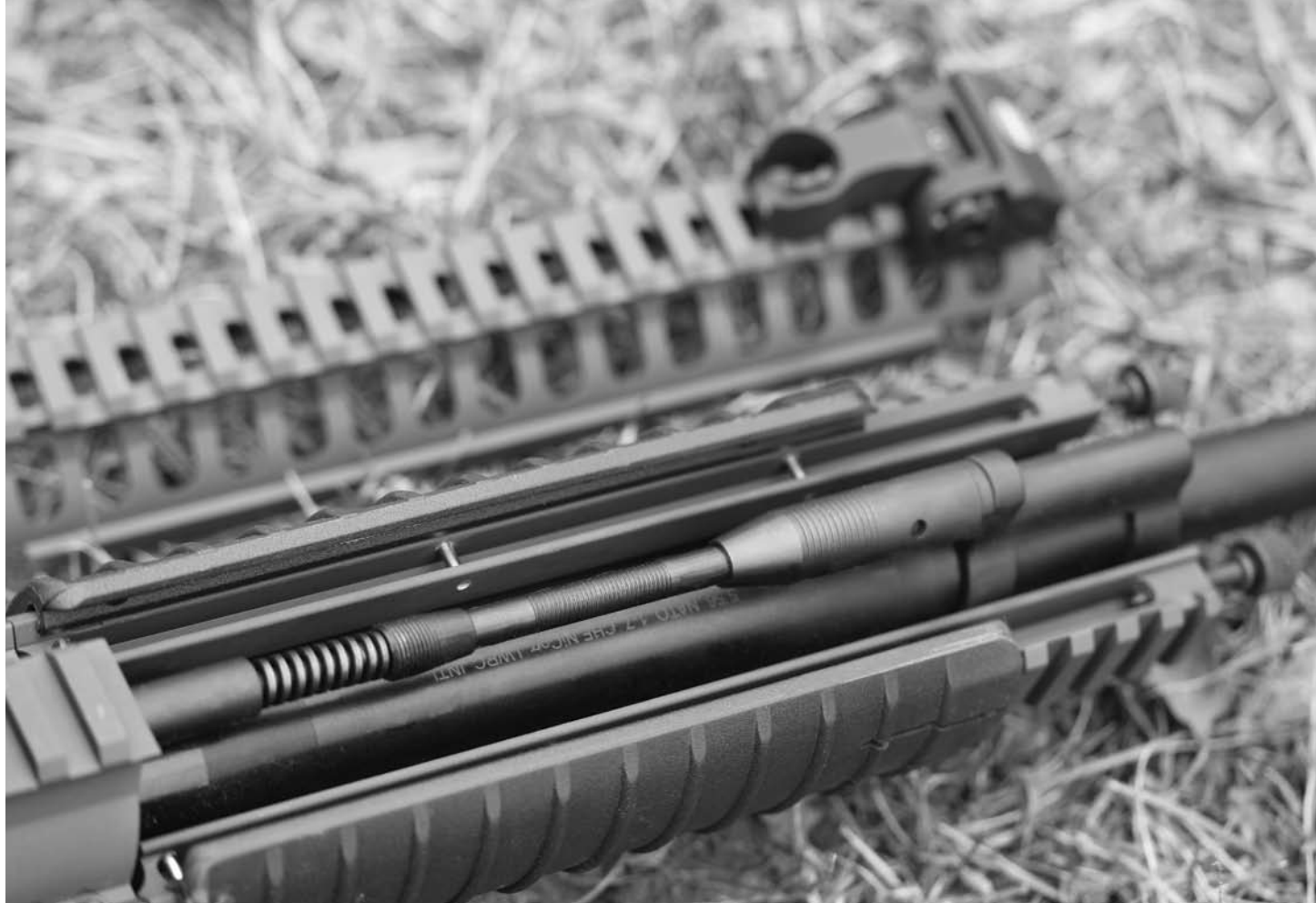
The LWRCI piston system: a short-stroke with a piston that travels farther than the M1 Carbine, but is not as lengthy as the Garand.
